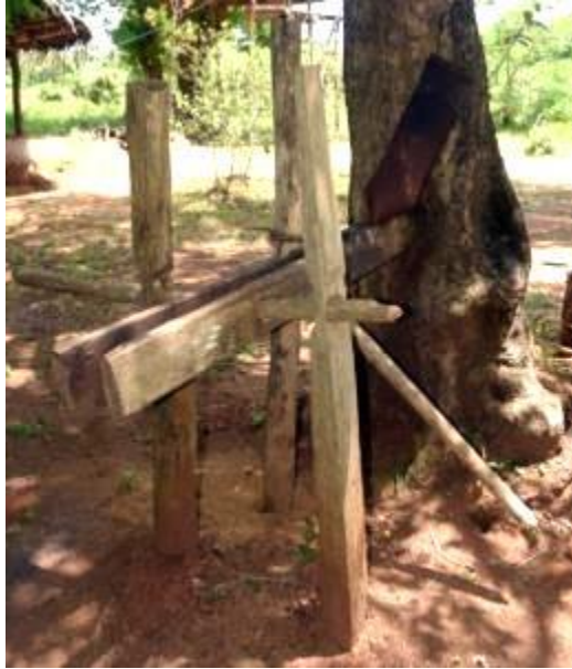
Figure 35: Pas pattalaya (for extracting oil from mee seeds), Palugaswewa
