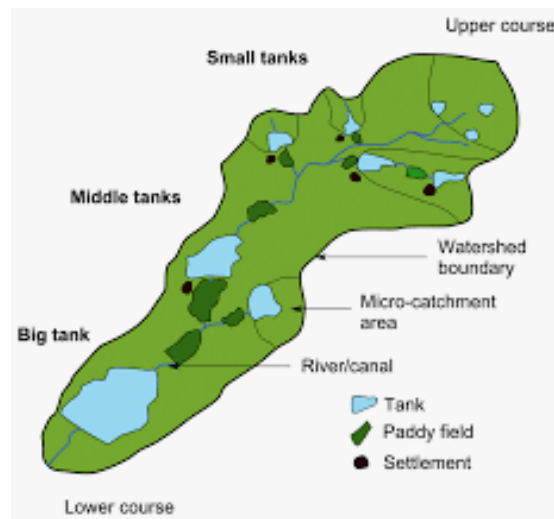
Figure 3: Schematic representation of a tank cascade system (Source: Brigitta Schütt et. al. 2013)
